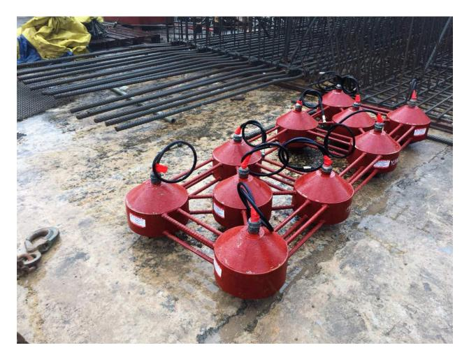
To illustrate the practical benefits of the BDSLT, we can examine its implementation in a real-world project. In a recent Mass Rapid Transit (MRT) project in Malaysia, the YJACK Bi-Directional Pile Load Test was employed to assess the load-bearing capacity of foundation piles.
