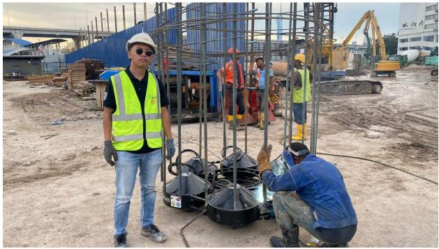
The YJACK Bi-Directional Pile Load Test represents a significant advancement in the field of static load testing. YJACK technology integrates advanced instrumentation and data acquisition systems to enhance the accuracy and efficiency of the BDSLT.
